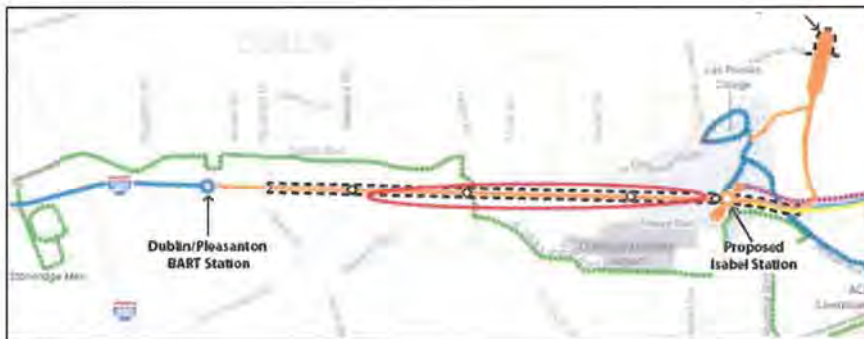
Figure 1. The red oval indicates the location of a Zone 7 pipeline along the south side of 580 between Santa Rita and Isabel Ave.; this could be impacted by the BART project dependent on how far to the south 580 would be widened to accommodate the BART tracks.
