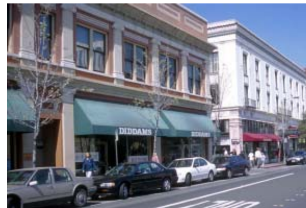
Windows are typically larger for ground floor retail uses than they are for upper floor uses.
