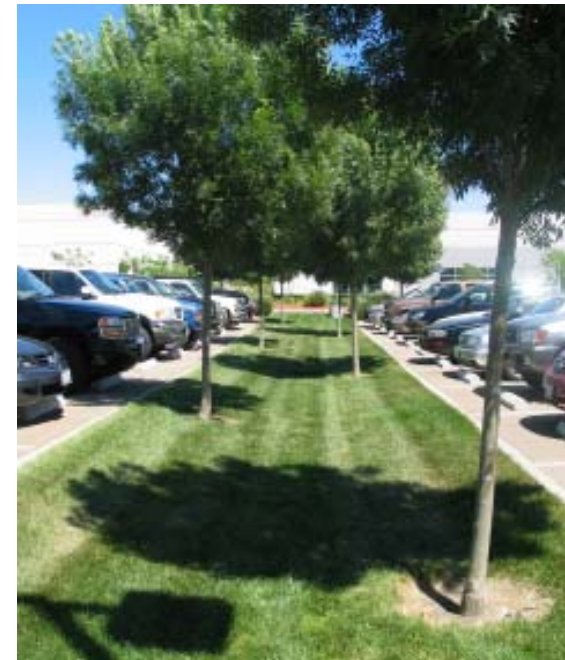
Drainage swales for parking lot run-off reduce negative impact on overall water quality.
